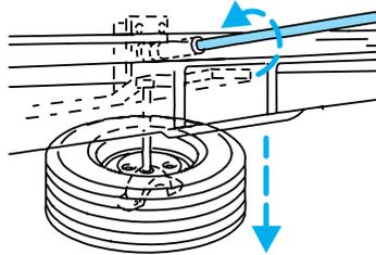
5. Remove the retainer through the center of the wheel.
