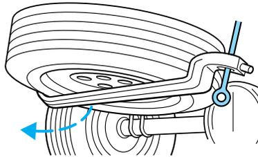
3. Insert the hooked end of the jack handle into the rear bumper opening.
