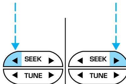
To set the minute, press and hold the CLK control and press:
