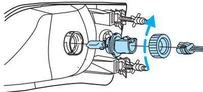
5. Without turning, carefully pull bulb out of headlamp assembly.
