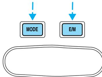
**Fuel range.** This displays the approximate number of kilometers (miles) left to drive before the fuel tank is empty. The indicated distance to empty may be inaccurate:
