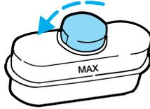
4. Use only a DOT 3 brake fluid certified to meet Ford specifications. Refer to *Lubricant specifications* in the *Capacities and specifications* chapter.
