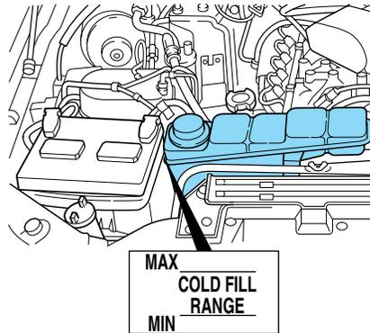
If the engine coolant has not been checked at the recommended interval, the engine coolant reservoir may become empty. If this occurs, add engine coolant to the reservoir. For more information on engine coolant maintenance, refer to *Adding engine coolant* in this chapter.
