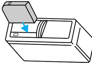
Radio power must be turned on to play the CDs in the changer. The magazine may be stored in the glove compartment when not being used. The CD magazine may be inserted or ejected with the radio power off.
