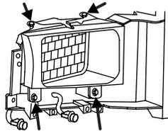
6. Remove the four screws and the headlamp retaining ring from headlamp.
